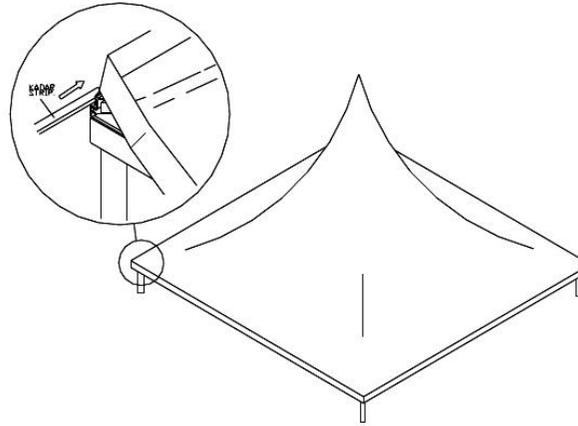
Fit Roof Keder into outer sail track on the side of the Eave Beam. Insert Kedar strip into the top of the roof in this same track.
