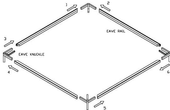
Lay out 4 x Eave Rails and 4 x Corner Connectors as above.
