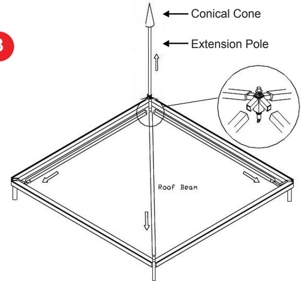
Insert 4 x Roof Beams to Corner Connectors then fit Roof Adjuster (make sure it is wound down to the lowest point).
