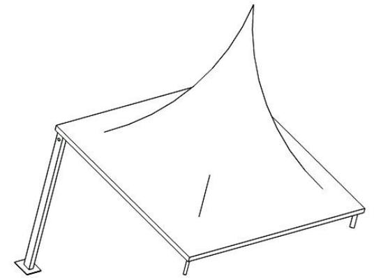
Fit foot plates to all legs using 2 or more people. Raise one side and fit 2 x legs. Fit extension pole and conical cone before fitting remaining legs.
