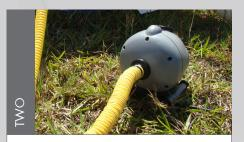
Connect pumps to inlet valves using the (IN) end of pump. Turn pump on and proceed to deflate using all 4 pumps.
