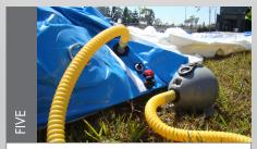
Connect all pumps to inlet valves using the (OUT) end of pump. Total of 4 pumps.
