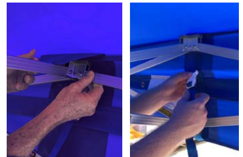
8. Ensure protective flaps are over the truss connectors. Attach them by looping the straps around the truss and engaging the clips, then tighten.
