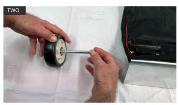
Insert the bolt through the wheel and bearing. Thread the nut until finger tight to secure the wheel.
