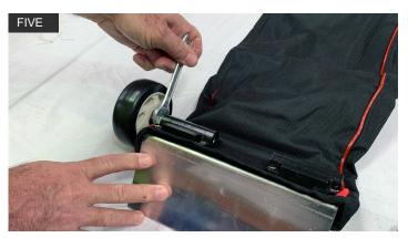
Tighten the nut on the inside of wheel until tight. **ENSURE WHEEL SPINS FREELY.**
