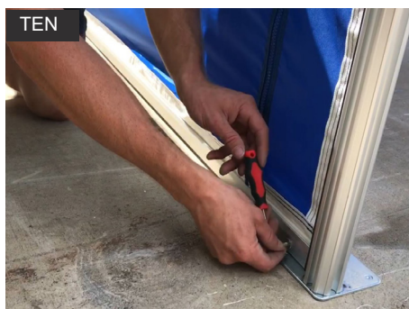
TEN Insert Bar connection into the tracking on frame. Adjust the Bar as need to be level and in desired position, tighten bolts to secure. Repeat.
