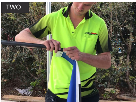
TWO Slide the Leg Rubber Inserts (2) along the Keda of the of the Wall Strips. Align to the bottom of Wall Strip.
