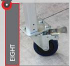
Set brakes to "off" position (do not stand underneath).
