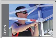
Pull all roof connector pins.
